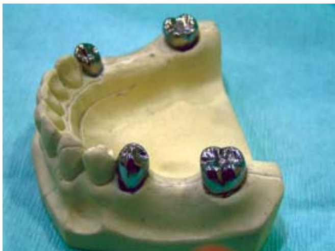
Fig 1: The experiment model with the four metal abutments showing the lines scored on the cast.
