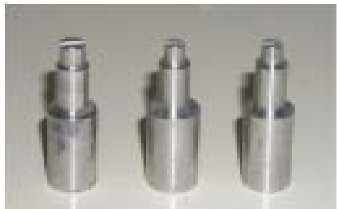
Fig 2: Master metal dies with different finish lines; From right light chamfer (0.5 mm, deep chamfer (1.0 mm); and shoulder (1.0 mm)
